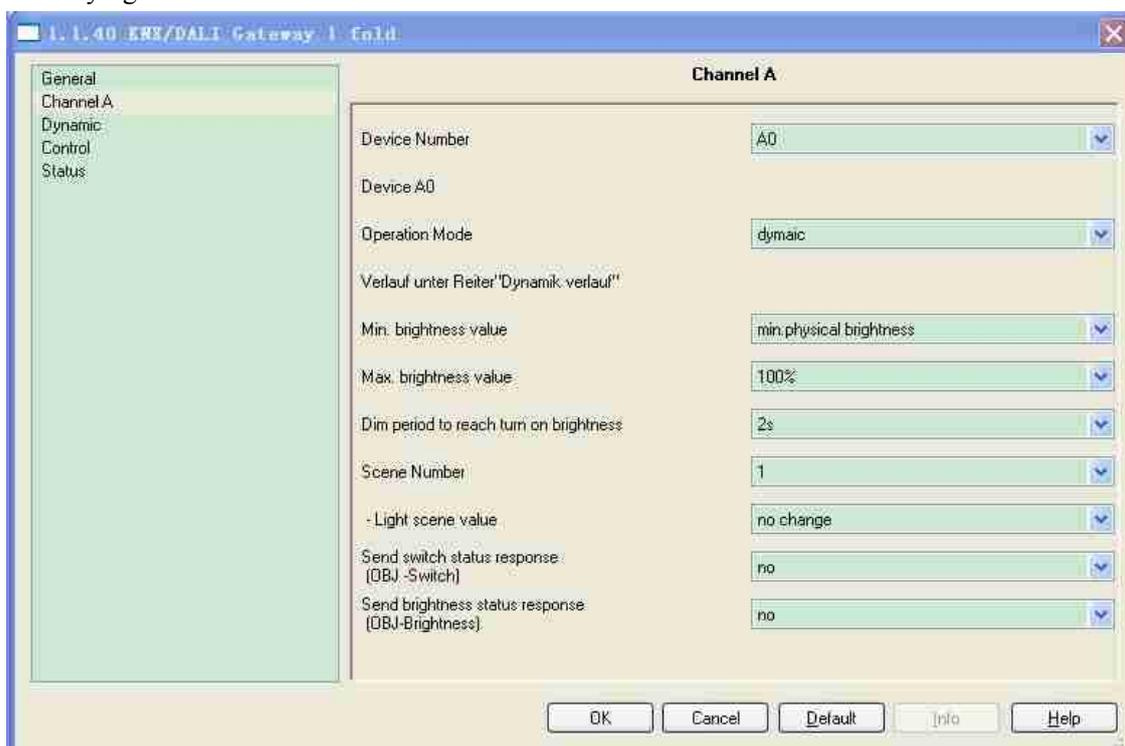
Figure 5.2 parameter settings interface " channel A" ( dynamic)
